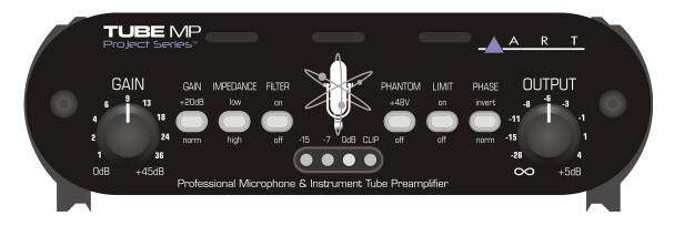
The **Gain Control** directly adjusts the input amplifiers giving you control over the dynamic range of your source. You get a 45dB range of control when using the XLR input and a 25dB range when using the ¼-inch input. Set the control counterclockwise to minimum gain when connecting the inputs.
