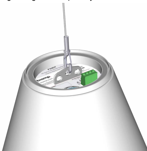
Figure 2. Attach primary cable snaphook in center hole
