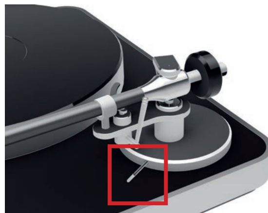
Pic. 9: Adjustment of the tonearm height
