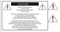
The lightning flash with an arrowhead symbol within an equilateral triangle is intended to alert the user to the presence of uninsulated hazardous voltage within the device's enclosure, which may be of sufficient magnitude to induce a risk of electric shock to persons.
