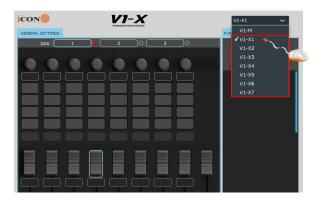
Step1: Connect the V1-X using a USB C connection. Ensure the latest iMAP is downloaded from the website and installed, (check to make sure your iMAP is up to date!). Run the iMAP.
