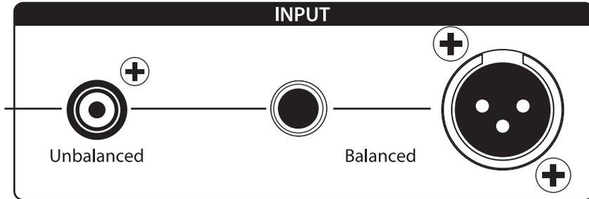
**Line-level Inputs.** The Eris Pro-Series monitors provide a choice of three line-level input types: balanced XLR, balanced 1/4" TRS, and unbalanced RCA. Do not connect more than one source to your Pro-Series monitors simultaneously.
