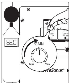
6. While measuring the output level with an SPL meter, begin slowly increasing the input sensitivity (volume) of your left speaker until the acoustic level of the test tone playing reaches 82 dB SPL. When both speakers play simultaneously, the overall SPL will increase by about +3 dB (85 dB).
