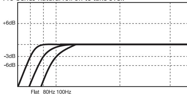
**Power User Tip:** If you are using a subwoofer that doesn't feature a variable low pass filter, like the PreSonus Eris Pro Sub 10 provides, you will use this control to set the crossover point for your 2.1 system. For information on configuring a 2.1 system in the studio, please visit [My.PreSonus.com](http://My.PreSonus.com).
