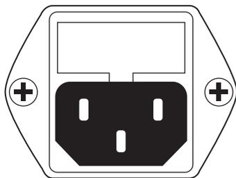
**IEC Power Connection.** This is the power inlet for your Eris Pro-Series monitor.
