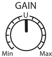
**Input Gain.** Sets the level of the input signal before it is amplified.
