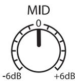
**Mid Frequency.** Boosts or cuts frequencies around 1 kHz by  $\pm 6$  dB.
