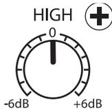
**High Frequency.** Boosts or cuts all frequencies above 10 kHz by  $\pm 6$  dB.
