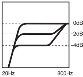
**Acoustic Space.** Cuts the level of all frequencies below 800 Hz by either -4 dB or -2 dB to compensate for the bass boost that naturally occurs when a speaker is placed near a wall or a corner. If your Eris Pro-Series monitors can be placed away from the walls in your mix space, leave this control set to 0 dB.
