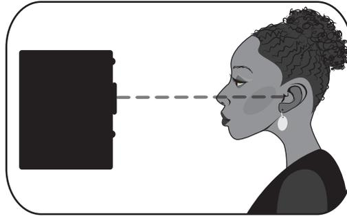
Ideally, near-field studio monitors like the Eris Pro-Series should be placed so that the high-frequency drivers (commonly known as ‘tweeters’) are at the same height as your ears when you are seated in the mix position.
