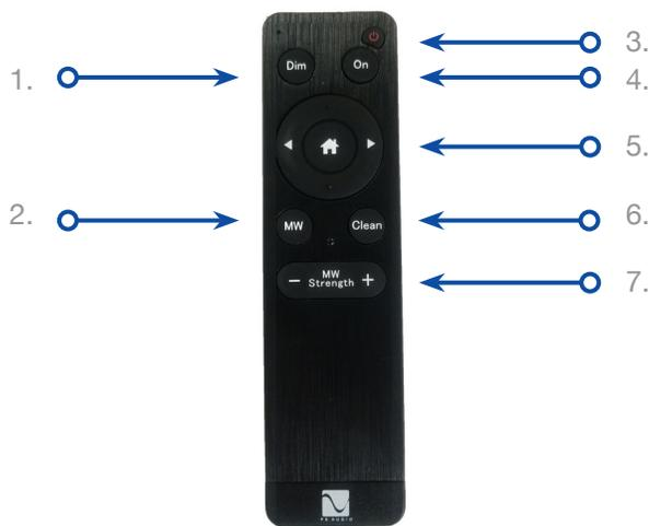
1. The Dim button turns the P20's display on and off.
