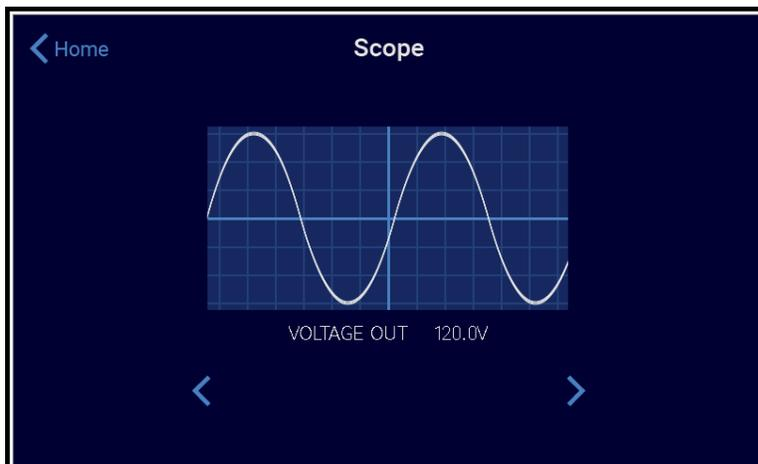
This is a fully functional oscilloscope that you can use to view the incoming AC waveform. Pressing either of the arrow buttons will scroll through the voltage in, voltage out, and the difference windows. In this way, you can see the degree to which the P20's output waveform is superior to the incoming AC sinewave.
