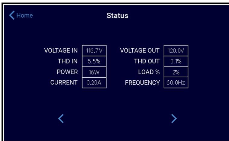
Here you can see the P20's overall performance data. Note how in the above image the THD output is significantly reduced and the output voltage is a stable 120 Volts. Press the Home button to return to the Home screen.
