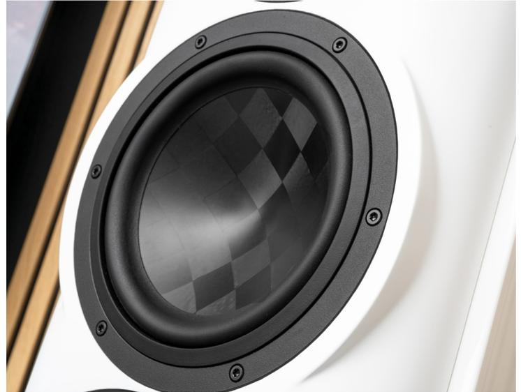
One of the two inner woofers. As with all four cone drivers, its cone is made of an extremely lightweight carbon fibre that is woven into a multi-layered yet thin-walled mesh. The lightweight and highly robust fabric enables high acoustic agility and impulse fidelity - and produces an attractive chequerboard look.
