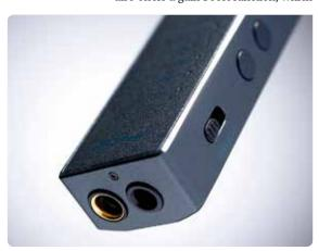
together with a notional max output 7.5v should drive most devices. There's also a special impedance-matching low-gain mode for sensitive earphones.
