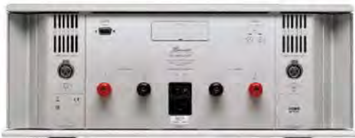
The final version has the minimum necessary configuration. The input end is only balanced, and number 3 is hot remains unchanged. Equipped with 1 pair of speaker terminals.
