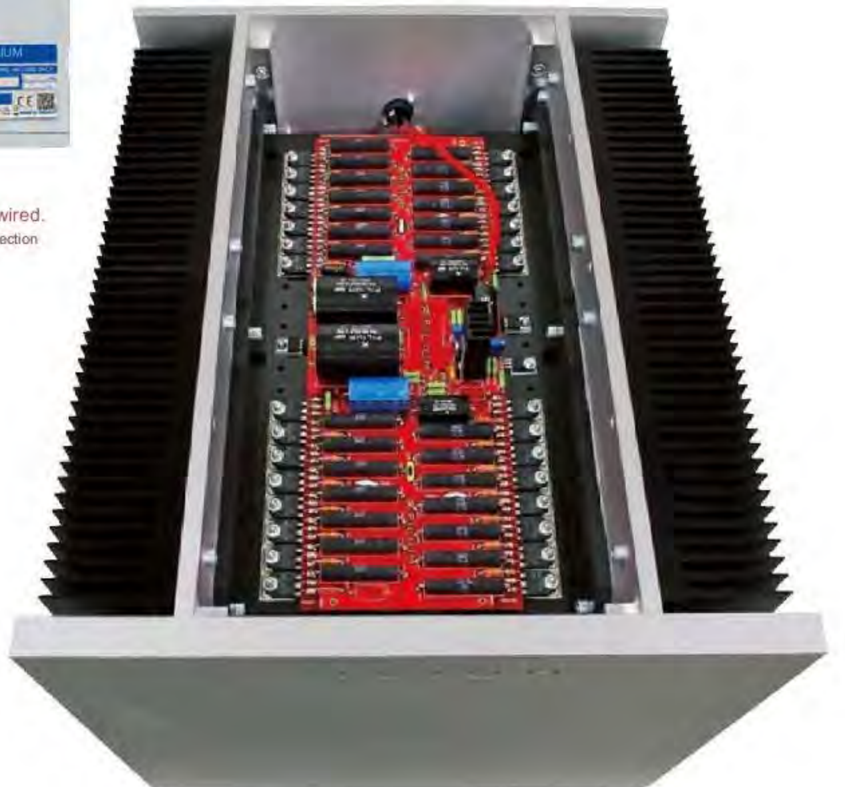
Inside the Hercules, the 14-parallel push-pull configuration Yamanki element stands out. Along with the casing, there is a super large 2.5kVA power transformer and a 24F. There are several filter capacitors installed.
