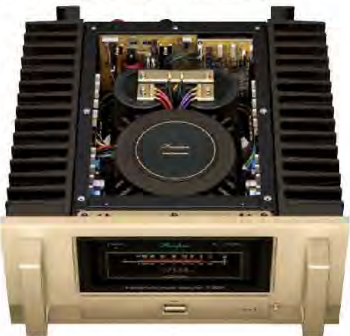
Peak inside. On the A250, the filter capacitor is in front and the power transformer is in the back. However, with this machine, the power transformer is located at the front, and the filter capacitor is placed at the rear. The output element MOS-FET is from Toshiba to Fairchild, changed to manufactured.
