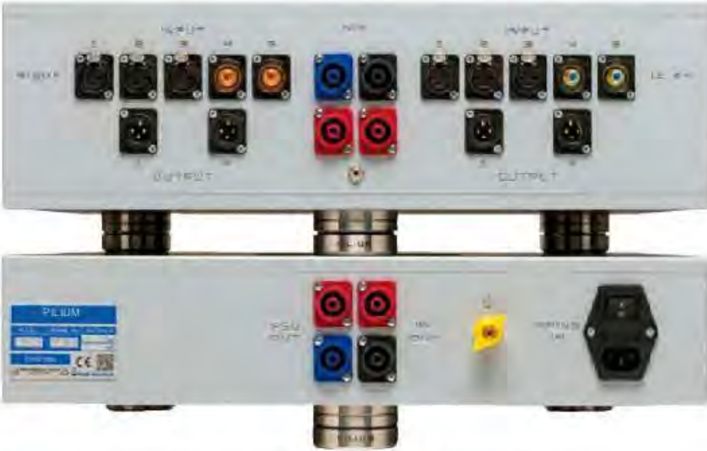
Alexander rear preamp. The main unit and the power supply are separate casings, and the two are connected using four Speakon cables. The main unit (top photo) has a panel layout for left and right channels, and has three balanced and two unbalanced input terminals. One of the two output terminals is balanced, and the other is a unique P-Link terminal prepared exclusively for connection with company machines.
