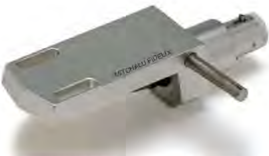
MITCHAKU" head shell connector part included with MC-F1000. At the top, the guide pin moves like a seesaw, allowing the tone arm to be in close contact.
