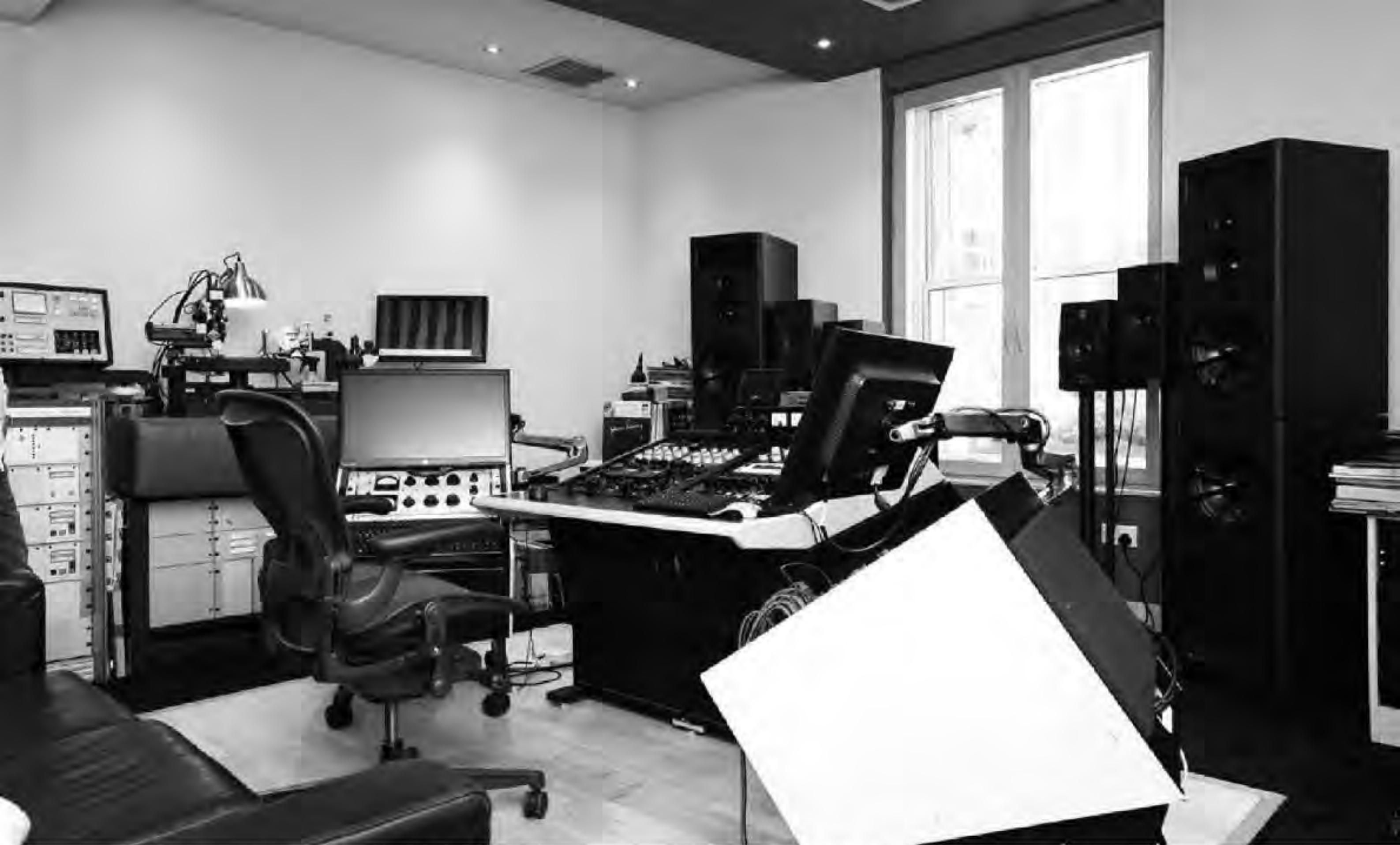
Mr. Showell's mastering room in Abbey Road Studios is set up with equipment selected by "Kanshin Ear", and the monitor speakers are PMC's, which he trusts today. We use the active type "MB2 XBD" (a 3-way configuration device equipped with two 31cm diameter woofers).
