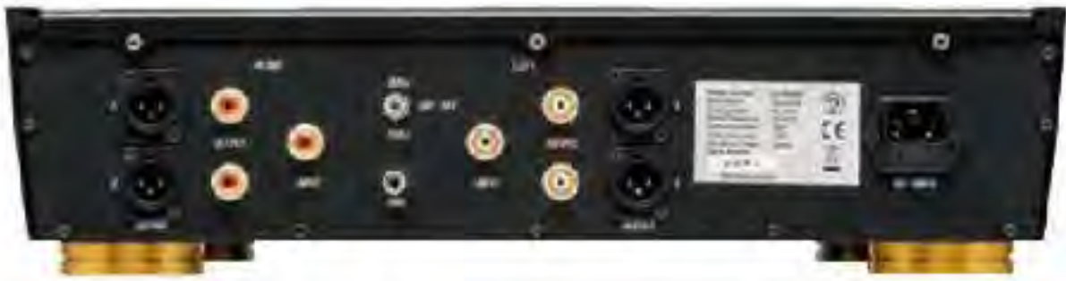
The rear of the DS-W3 equalizer has one optical cartridge dedicated input terminal and an ultra-low One system each of balanced/unbalanced output terminals with different cutoff values. Output 1 is equipped with a 6dB/oct filter, output 2 is 12dB/oct. 30Hz/50Hz cutoff frequency switch at the top center. A total of 4 patterns when combined with It is possible to set ...
