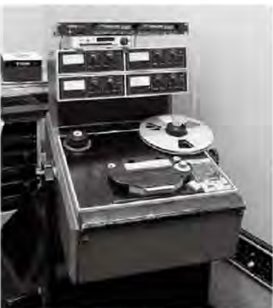
I use an Ampex to play analog tapes. "ATR102 | Open reel deck:"
