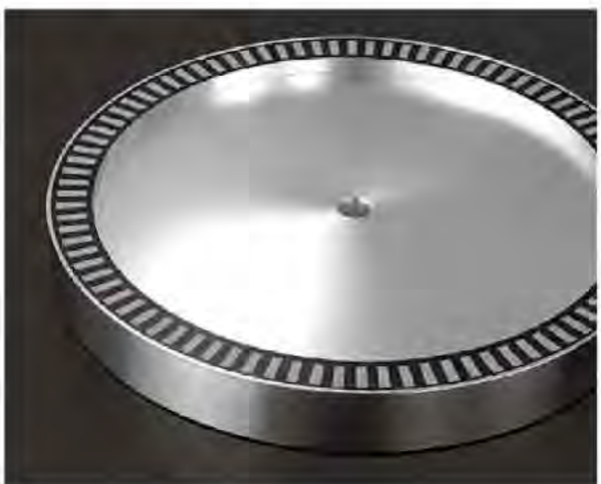
A 300-diameter platter machined from an aluminum block and machined with precision machining. Thickness: 35 mm, weight: 5.2 kg. A strobe pattern with a striped pattern is engraved on the outer periphery of the back of the platter. It is.
