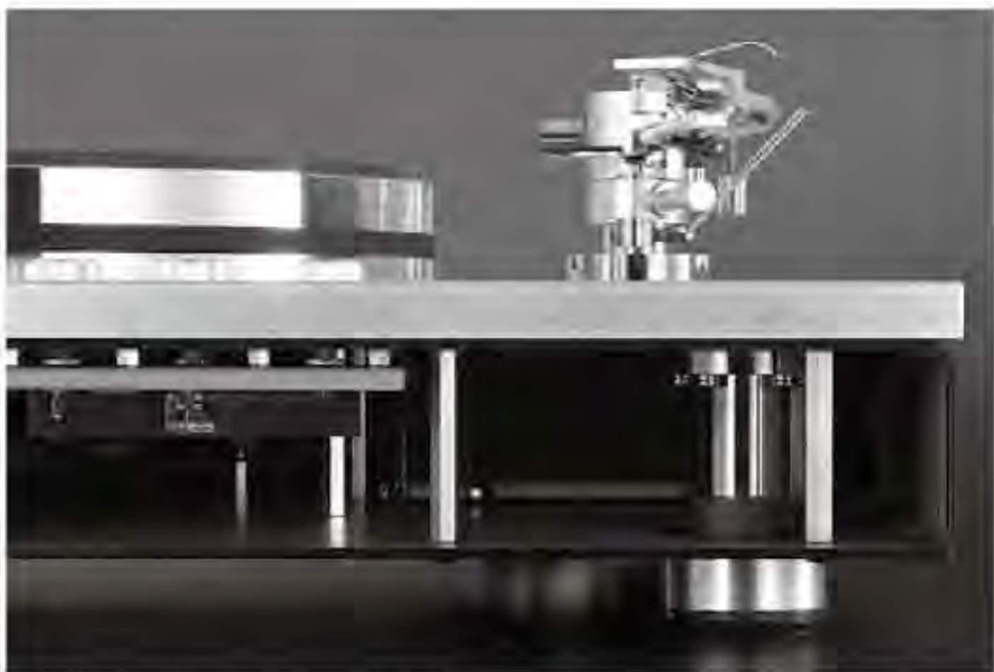
The main parts (spindle, platter, tone arm) are attached to a 15mm thick top plate, and an underslung structure is used in which the main parts (spindle, platter, tone arm) are connected to the ground through the control insulator legs. In addition, by floatingly mounting the drive motor and power transformer on a newly installed 3.2mm thick bottom chassis via vibration damping rubber, the signal pickup mechanism is separated from the vibration line, resulting in mechanical S/N (rumble). Improvements have also been made in howling performance.
