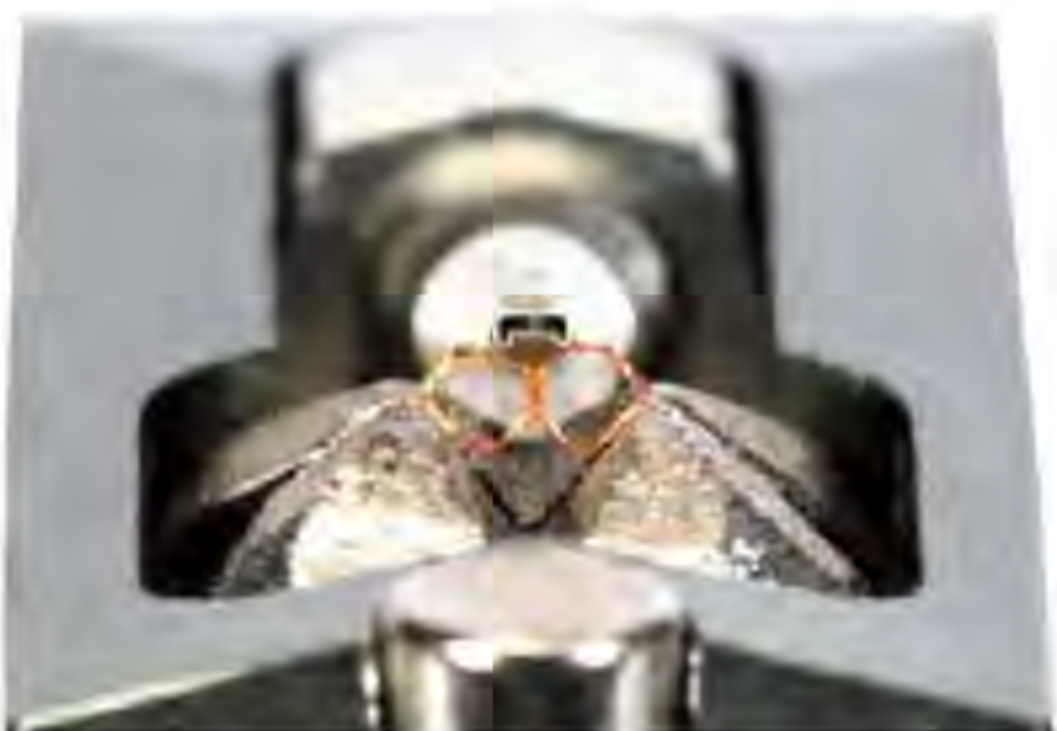
Close-up of the cantilever tip. A coil with a diameter of approximately 0.8 mm is at the tip of the needle. Adopts a direct coupling type arranged in two parts, not circular. The pentagonal coil increases stability against shaking and twisting.
