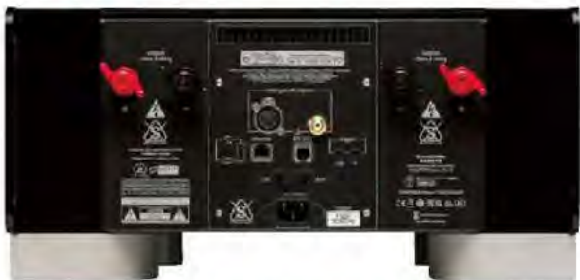
There are 2 speaker terminals. It has one unbalanced and one balanced input system. There are also RS232 for centralized management, Ethernet, and a USB port for internal software updates. The sole is an isolation foot with an internal structure to reduce vibration.
