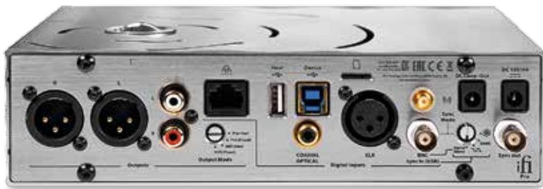
ABOVE: Digital inputs are shared across a combined coax/optical socket (S/PDIF), USB-A and B sockets, AES/EBU (on XLR), micro SDHC and wired/wireless Ethernet. A multifunction BNC input also accepts external clock sync'ing. Balanced (XLR) and single-ended (RCA) analogue outputs are configurable as either fixed or variable
